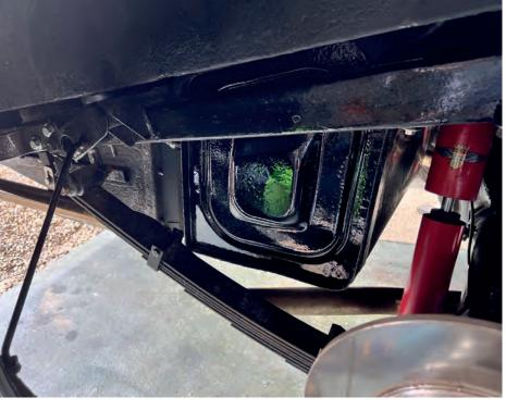
While the engine was out we were able to thoroughly inspect the chassis and all the inner wing areas, including the battery boxes. To our delight, the chassis was in incredible condition and we had to make the decision about removing the body or leaving it on.
