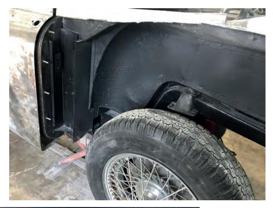
• Left and below: POR-15 applied. The underside of the car was thankfully in surprisingly good condition, although a cracked rear spring was discovered during the disassembly process
