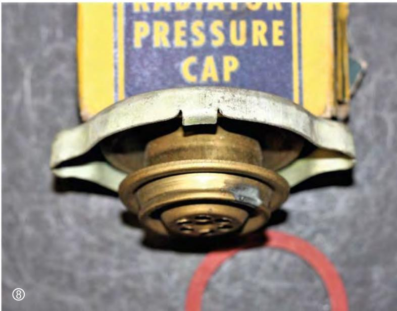
The closed-type radiator cap has a valve housing that contains both the over- and under-pressure relief valves. When the bayonet cap is screwed down on the radiator neck, this valve housing is firmly pressed against a fibre washer at the bottom of the radiator neck, which seals the cooling system. So this separate fibre washer is not a part of the cap but is often held in place by a number of 'dimples' positioned at the circumference of the radiator neck to prevent the fibre washer getting lost.
