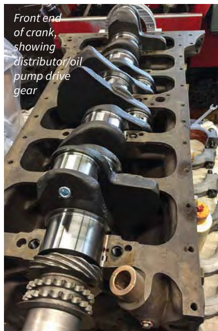
Crank installed with new seal housing behind the flywheel end
